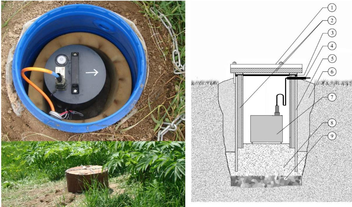
**Figure 2.** Equipment installation seismometer module (1. Module cover; 2. Heat insulation; 3. Sealing ring; 4. Input signal cable; 5. Module housing; 6. Filling; 7. CME-6111 seismometer; 8. Concrete base; 9. Crushed stone).
