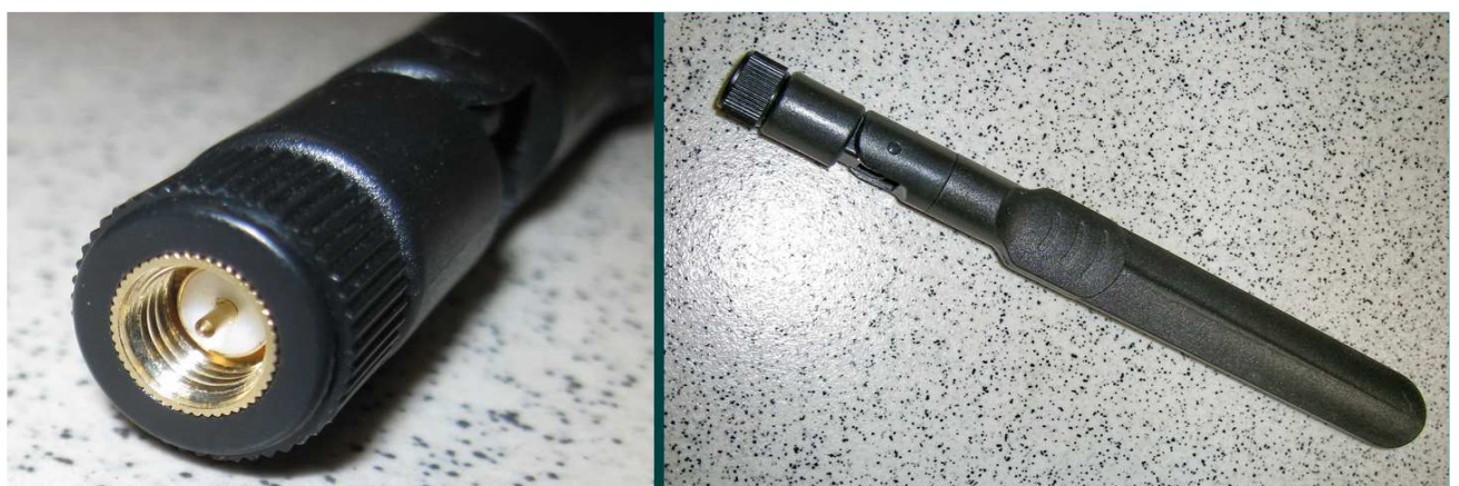
Fig. 6. Wi-Fi antenna – connector view
