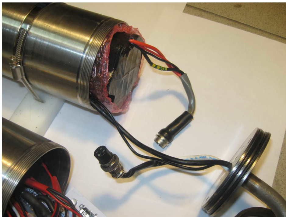
Fig. 10. The battery's installation
