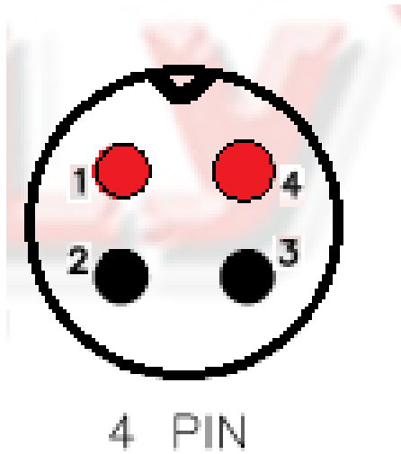
Fig. 4. The battery connector pinout (Male connector, front (pins) side view)
