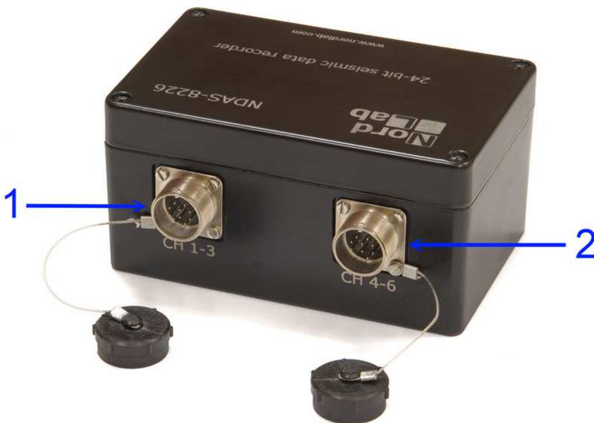
Fig. 1. The seismic sensors connectors
