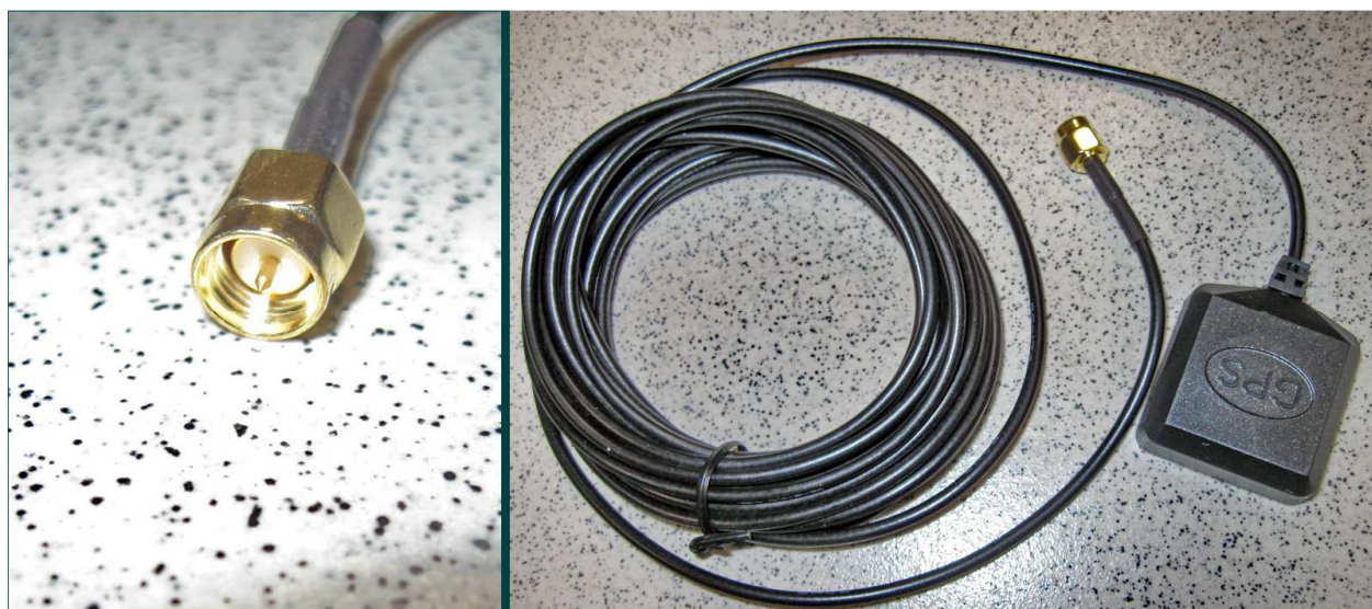
Fig. 8 GPS Antenna, connector and appearance
