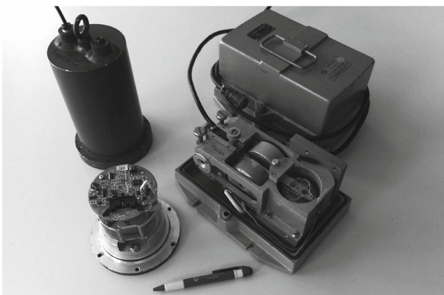
Fig. 2. SM3-OS pendulum seismometer with removed cover (right), seismometer based on molecular-electronic converter, and airtight box for marine studies (left).
