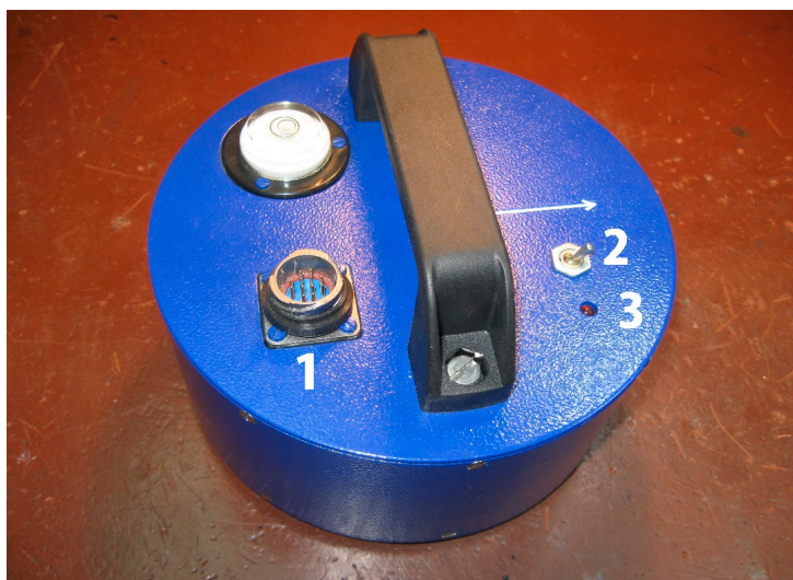
Figure 11. Combined sensor. Marked are output connector (1), MEMS switch (2), MEMS state indicator (3).
