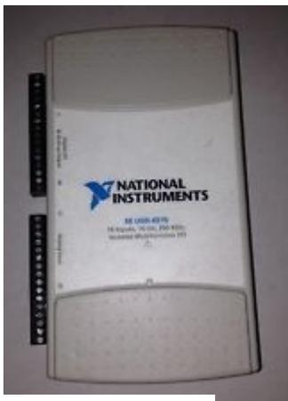
The NI USB – 6215 unit is used for the calibration digital control in case of this option is used.
