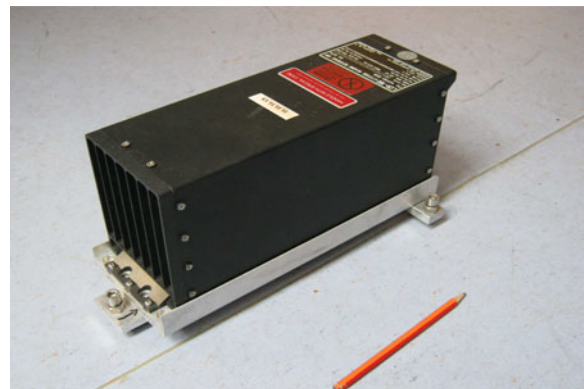
Fig. 2 The LCG-Demonstrator can measure three components of rotation with three orthogonally aligned fiber optic gyroscopes and three components of transverse acceleration using three silicon MEMS accelerometers
