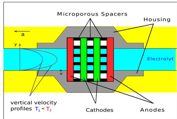
**Fig. 1** The measuring device in the liquid-based rotational seismometers R1 and R2 is an electrochemical transducer consisting of two platinum mesh anodes and two platinum mesh cathodes that are sandwiched between micro-porous, isolating spacers (after Eentec 2006). The current of ions through the transducer depends on dynamic viscosity and thereby on the fluid temperature
