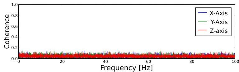
**Fig. 4** The coherence spectra for all three rotational components of the LCG-Demonstrator (S/N 2056 and 2276) show that the contribution of coherent ambient noise sources was very small during the self-noise measurements
