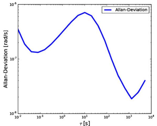
**Fig. 9** Allan deviation of the R1 (Z-axis); similar to the R2 sensor the form of the Allan variance in the period range from 0.1 to 1,000 s might be related to non-linearity of the transfer function of the instrument in this period range
