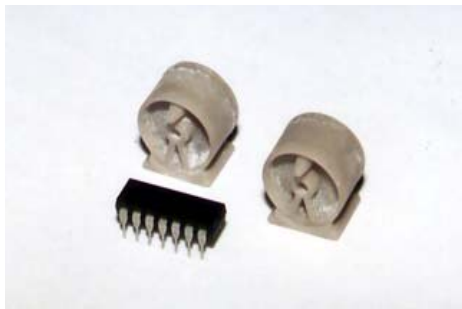
Fig. 6 Example of the molecular-electronic linear accelerometer.
