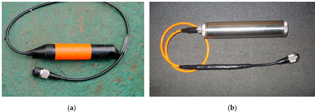
Figure 6. Hydrophones. (a) Reference hydrophone at GS-PV-1S; (b) molecular-electronic transfer (MET) hydrophone.
