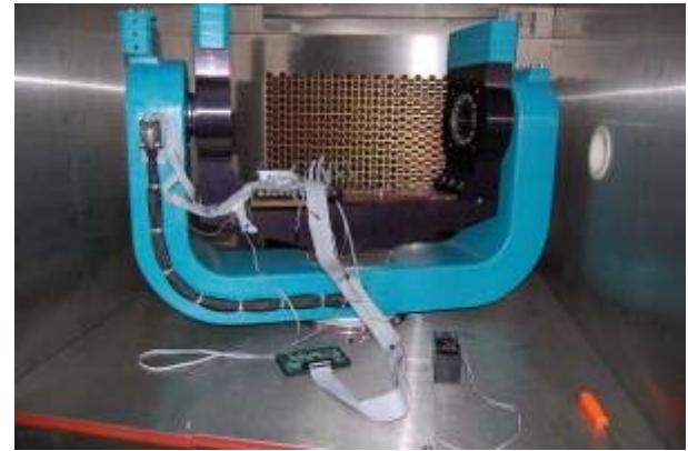
Fig. 4. One-axle motion simulator ST1144C with thermal camera 750T30/4 Climats in the horizontal position with 3 rotative and 3 linear components fixed for technical parameters testing.
