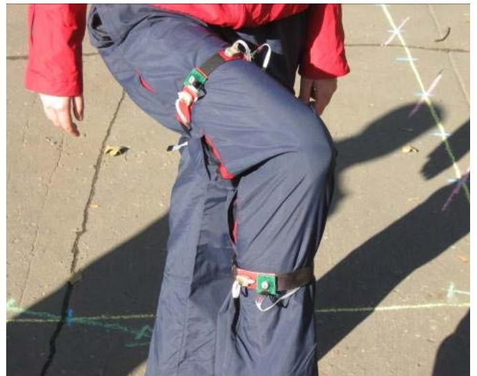
Fig. 9. Angular motion and linear acceleration sensors fixed on foot of the examiner
