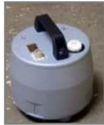
Seismometer CME-4111-LT (a low temperature model)
