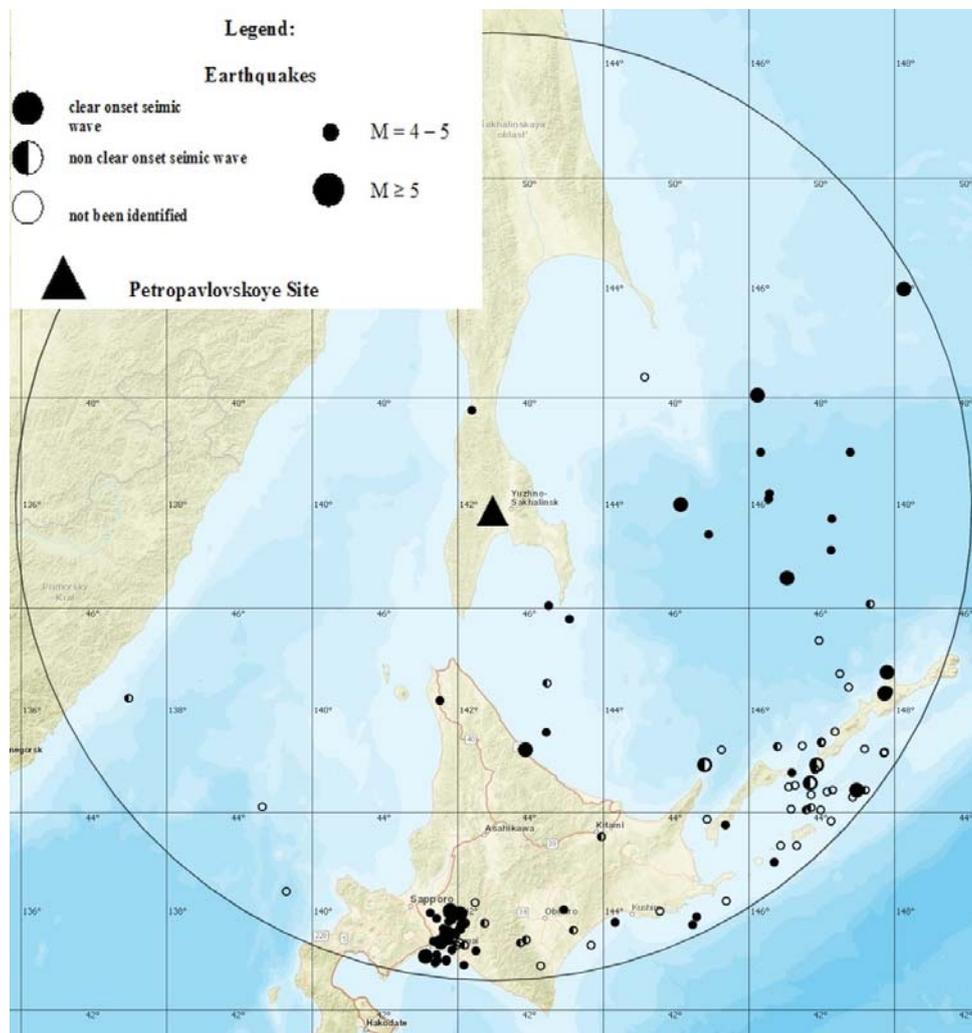
**Figure 6.** The map of earthquake epicenters, based on the analysis of the operational catalog of the SB GS RAS with  $M \geq 4$  (June-September 2018) by the seismological complex CME-6111+ NDAS-8226.
