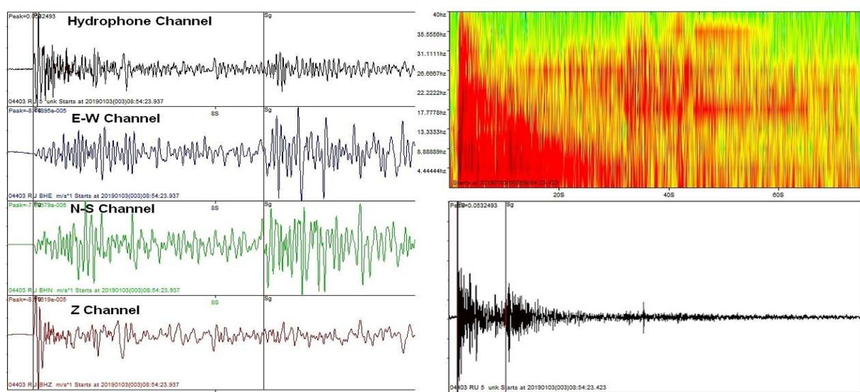
**Figure 5.** Recording a local seismic event with molecular electronic sensors. To the right is the spectrogram of this event, recorded by a hydrophone.
