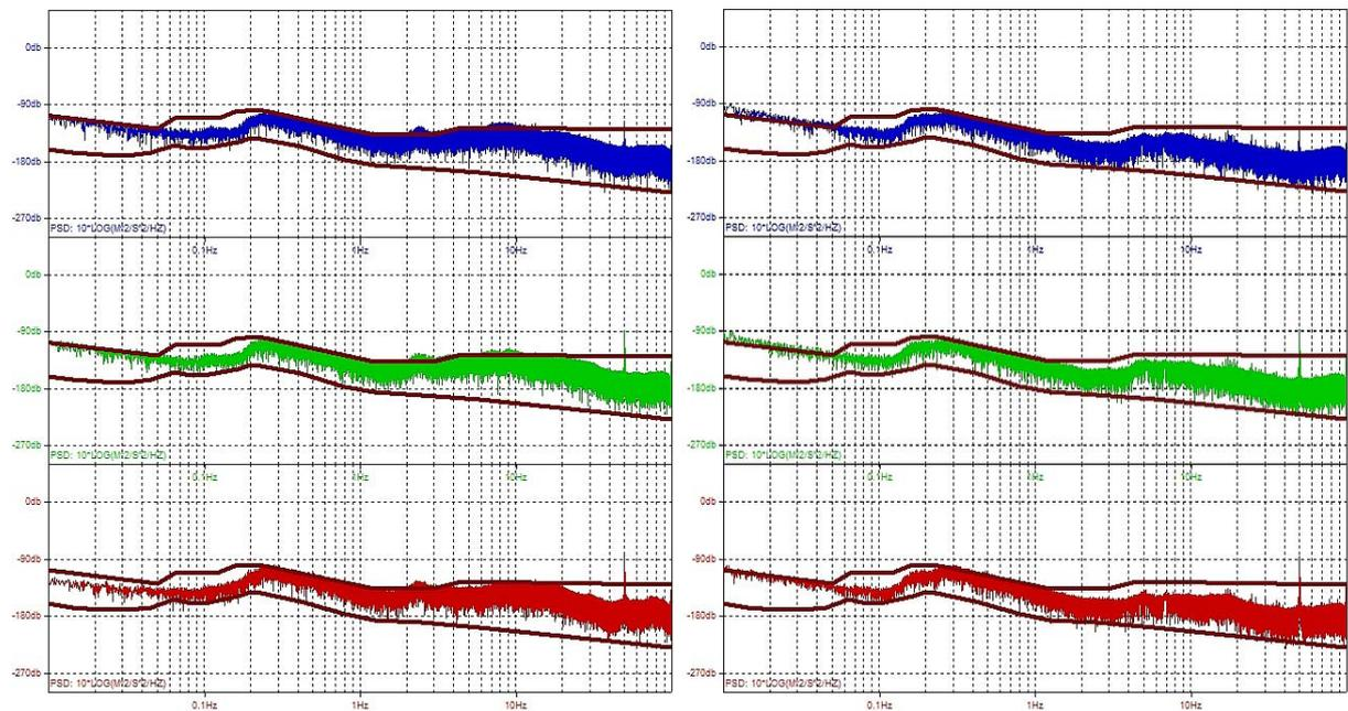
**Figure 4.** The spectral density of seismic noise of the CME-6111 seismometer (on the left - daytime, on the right – nighttime).
