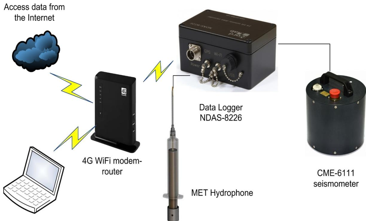
**Figure 3.** Equipment for seismic monitoring complex.
