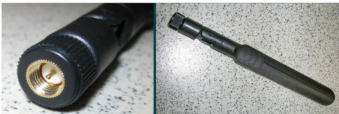
Fig. 4. WiFi antenna, connector
